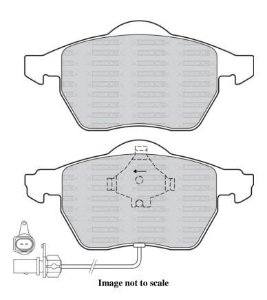
The inner (piston side) pads are often fitted with backplate springs that are offset, by about 2mm, relative to the centre line of the pad. Where pads are supplied with offset springs, the inner pads are not interchangeable and must be fitted to the correct caliper.
